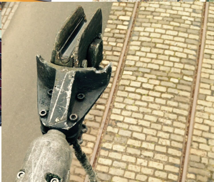
18 53's Trolley. The carbon slide nearing renewal after 6 years labour.
