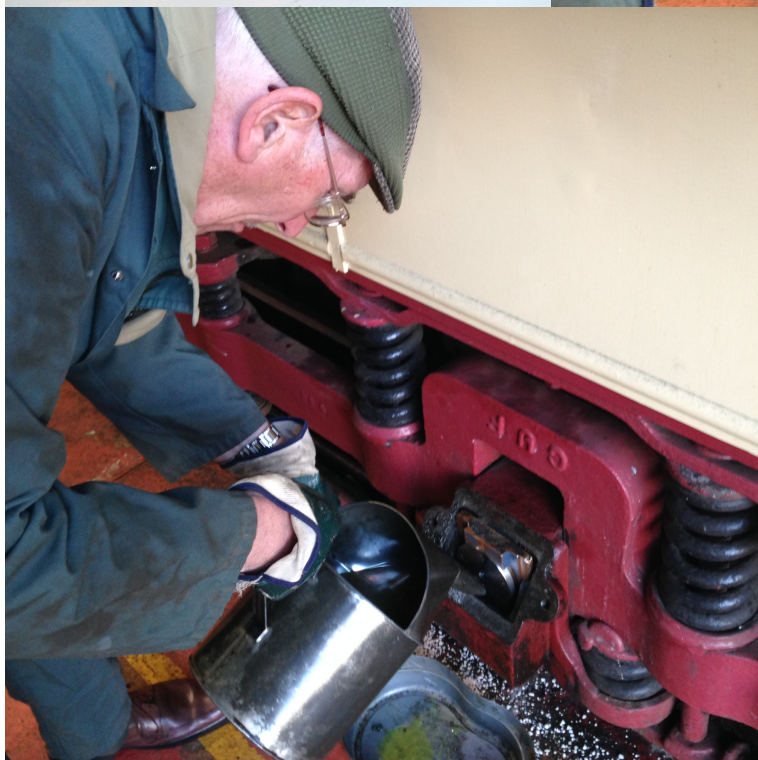
George Murray lubricates 53s axles
